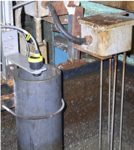
EchoPod Measures Level in a Stand Pipe
