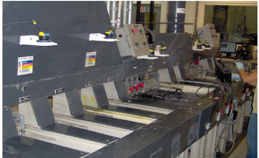
EchoPod Mounted in a Plating Tank
